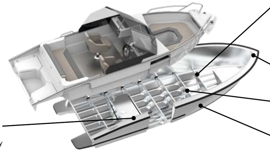
Reinforcing beams and strengthening cross sections in the hull, gives the boat exceptional torsional stiffness.
